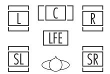
These indicators are the L/C/R/LFE/SL/SR letters that are inside the center boxes of the **Speaker/Channel Input Indicators** 14 in the front panel **Main Information Display** 23.
